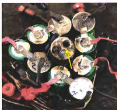
Figure 1. Photograph of the 10S1P battery post-propagation test showing the penetration of Cell 6.
