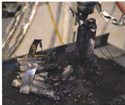
Figure 8. Photograph of the 1S10P battery post-propagation test.
