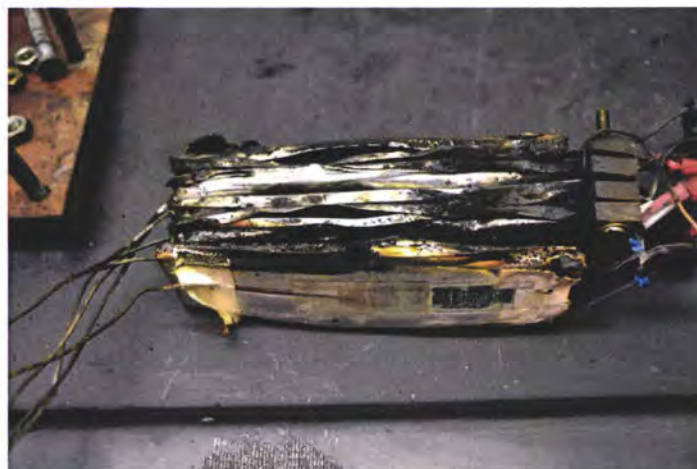
Figure 14. Photograph of the 5S1P battery post-propagation test initiated at Cell 1.
